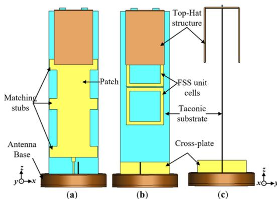
Fig. 6: High-gain printed monopole antenna
