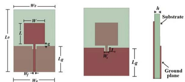
Fig. 5: Bio-inspired Printed Monopole Antenna
