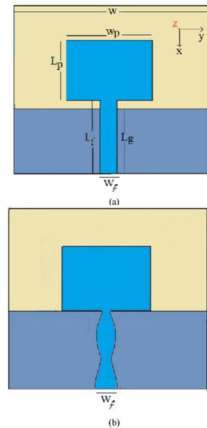
Fig. 4: Configuration of the printed monopole antenna
