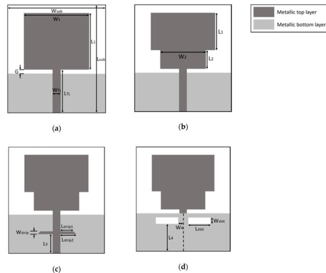
Fig. 2: UWB-Printed Rectangular-Based Monopole Antenna
