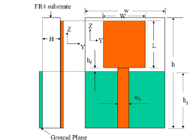
**Fig. 1: Geometry of the printed rectangular monopole antenna**
