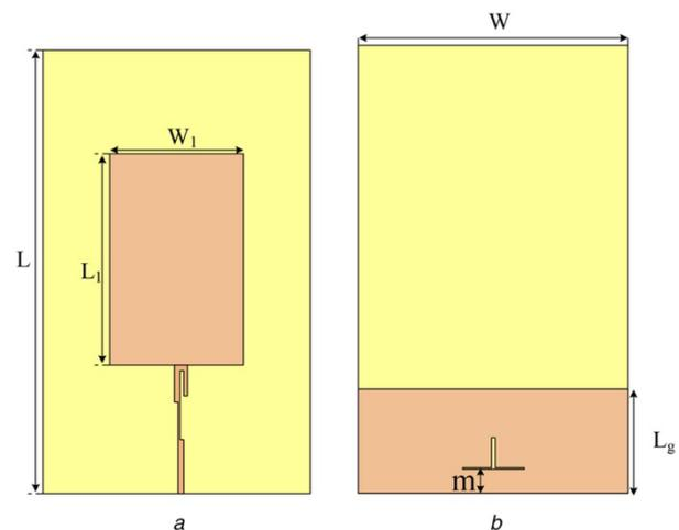
Fig. 7: Bandwidth enhancement and size reduction of printed monopole antenna
