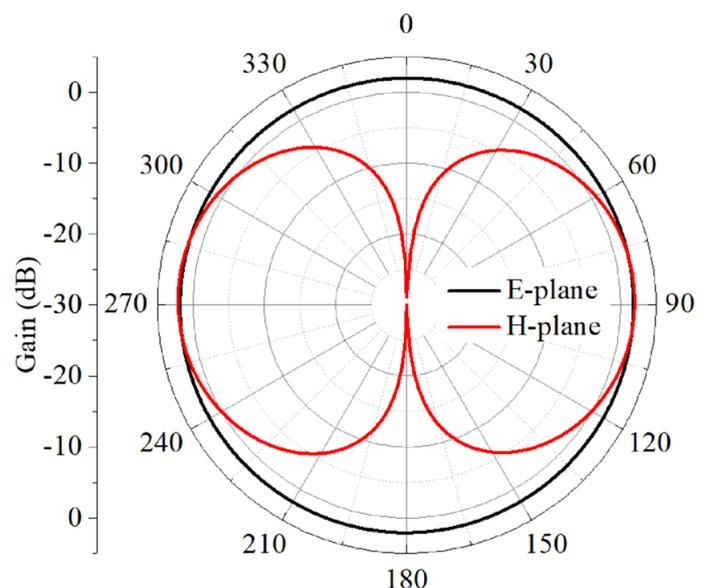
**Fig. 9: Monopole Antenna Radiation Pattern**
