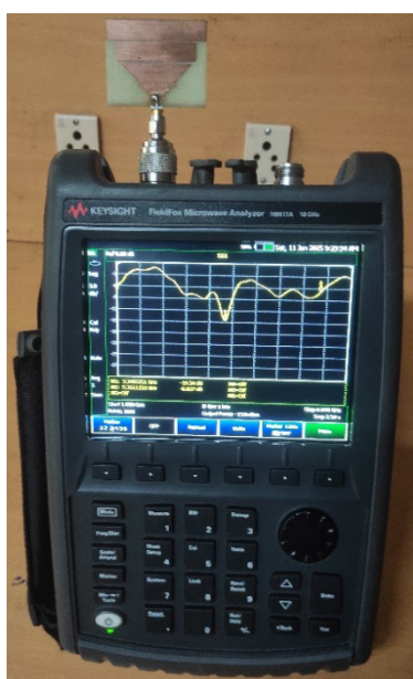
Fig. 6: The proposed MTTs Antenna with experimental setup
